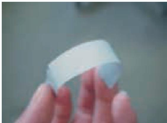
Fig. 1 Al-Ti-Fe powder sheet
